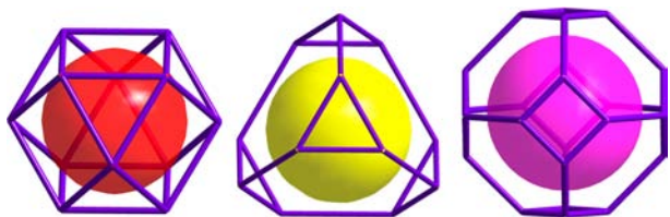
Figure 1. Schematic representation of the cuboctahedron (Cage A, left), truncated tetrahedron (Cage B, middle), and truncated octahedron (Cage C, right) existing in rht-type MOFs based on copper paddlewheel [\text{Cu}_2(\text{COO})_4] building blocks and C_3 -symmetric hexacarboxylate linkers.
